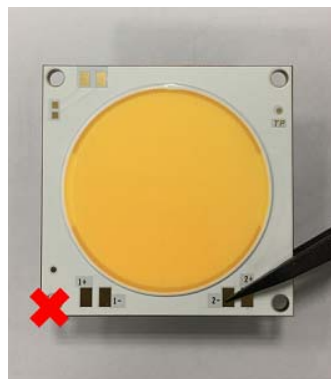
不可夾電極處 Don't clip both electrode
