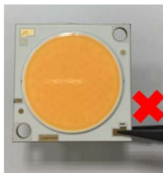
不可夾電極處 Don't clip both electrode
